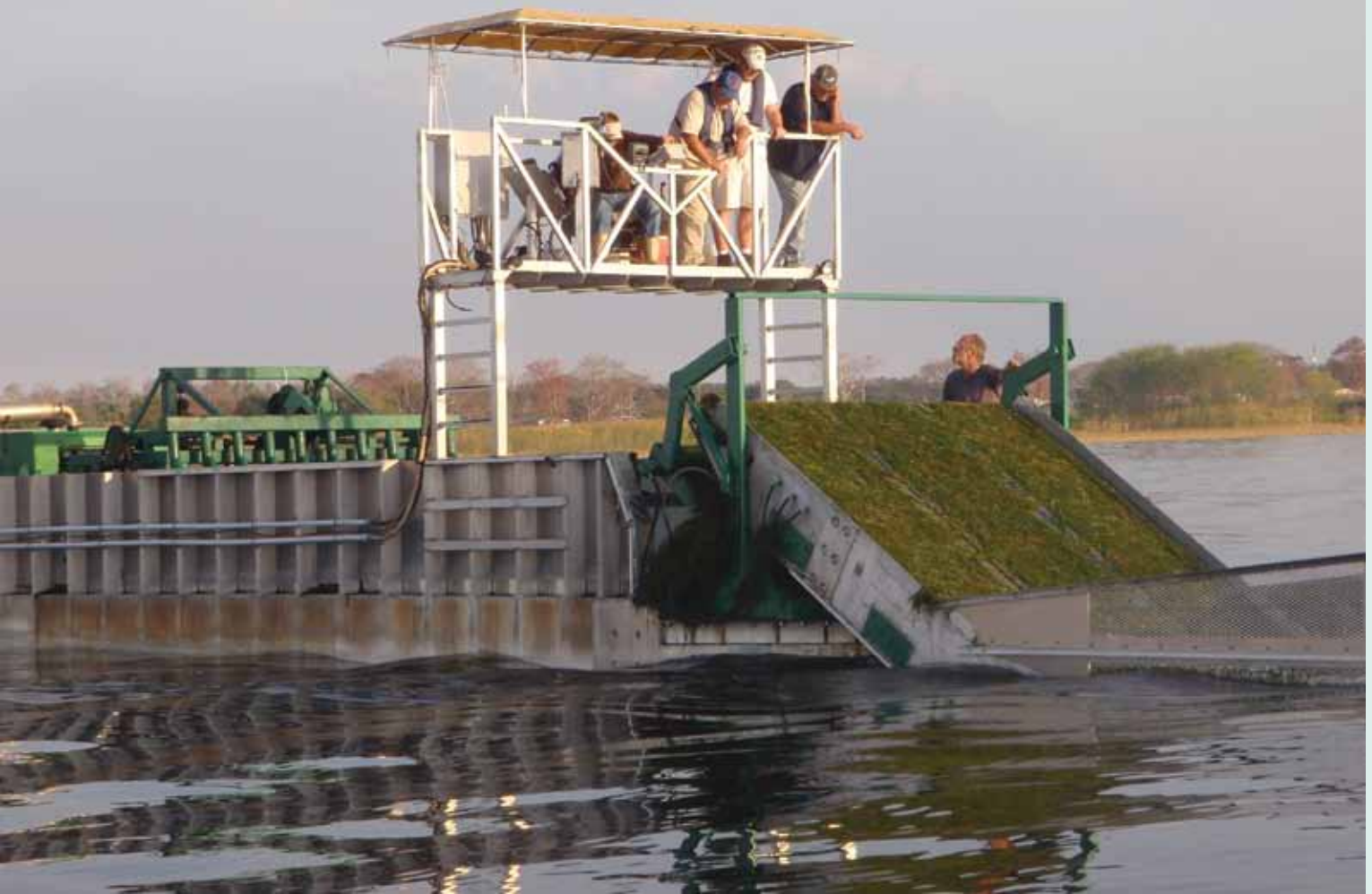
The 70 ft Kelpin Harvester was fitted with GPS navigation and the pickup table extended in order to harvest to a maximum depth of 10 feet, although most of the hydrilla in the Lake Toho site was only 3-6 ft tall in 8-9 ft of water. Photo by Dean Jones.
